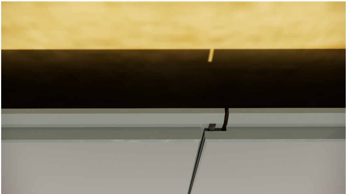
Option 3: Using panels slotted on all four sides
